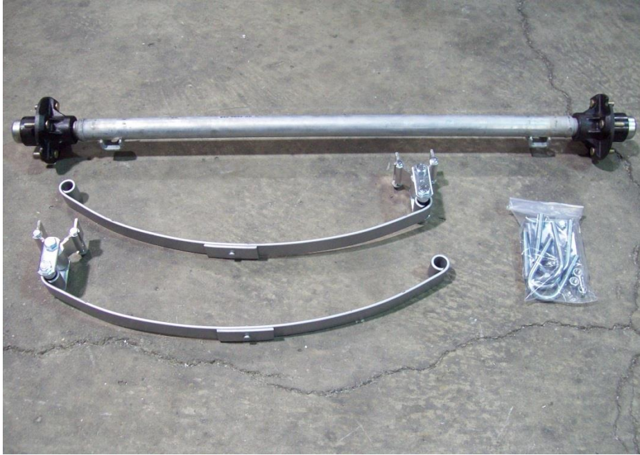
Axle, spring assemblies and U-bolt hardware.
